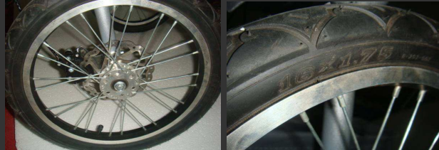
b. alloy rims with quality and thick tires 16"x1.75
